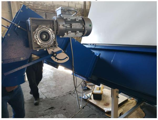
Installing the grain level sensor.
